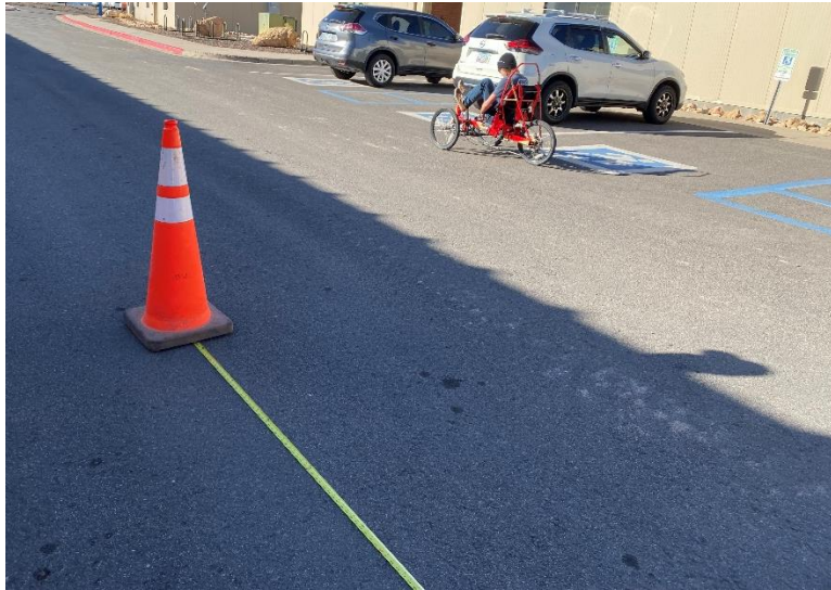
Figure 3 - Brake Distance Test Apparatus
